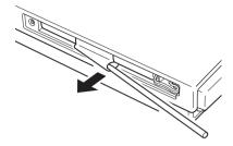
**4** Grab the extracted tape and partially pull the battery out of the unit.
